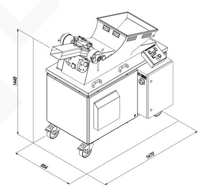
Butter homogenizer SHG is designed to rework bulk butter before re-packaging. Homogenizer SHG can be used with any butter filling and wrapping machine. Homogenizing is necessary to regain butter properties as they were before long storage or deep freezing. When butter is homogenized, it is ready again for packaging into customer size portions.
