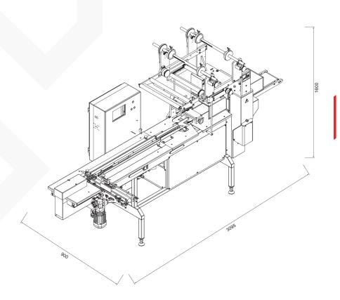
PM is a horizontal Flow-Pack type machine. Packs are sealed on three sides from a roll of heatsealable packaging film. It is compatible with AR2T curd filling and wrapping machine.
