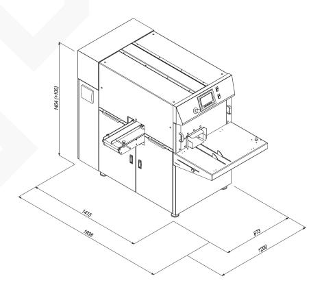
DSU is a semi-automatic cartoning machine used for grouping and stacking of butter bricks. Bricks are packed by ARM or any other filling and wrapping machine. It serves as an exceptionally reliable and cost-effective end of the line solution. Case packer operates at capacity of up to 100 bricks per minute. Different box sizes are possible.
