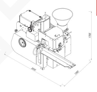
Curd filling and wrapping machine – AR2T is designed to fill and wrap curd (tvorog) into aluminum foil or parchment paper. Filling and wrapping machine AR2T could be used in combination with Flow-Pack machine PM.
