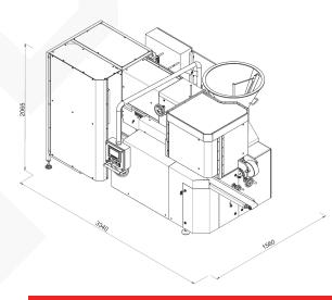
Processed cheese filling and wrapping machine is ARU an automatic packaging machine for foiling of processed and cream cheese with aluminum foil with or without easy opening system and labeling.
