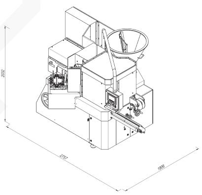
AR6U automatic packaging machine for foiling and heat-sealing of processed cheese with aluminum foil and packing into individual carton.
